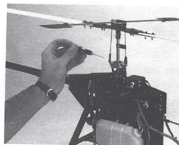
Apply a light drop of oil to each ball link and swashplate O-Ring.
