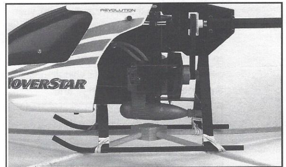
Proper HoverGuard attachment (not muffler clearance)
